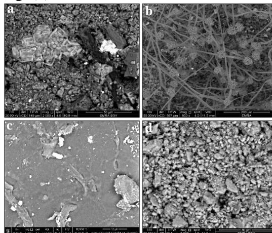
Figure (7) Shows SEM investigated samples before applying stains, **a.** salt crystallization on samples before applying stains, **b.** fungi stain, **c.** Sample after cleaning by nano gel, **d.** sample after cleaning by nano manetic gel.
