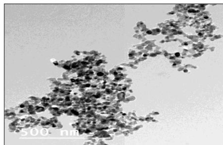
Figure (4) Shows a TEM image of iron nanoparticles biosynthesized by *Penicillium commune* MH5 filtrate
