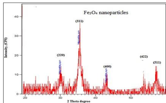
Figure (3) Shows XRD pattern of the iron oxide nanoparticles biosynthesis from  $\text{FeCl}_3$  treated with culture filtrate of the fungus *Penicillium novoparasiticus* MH5
