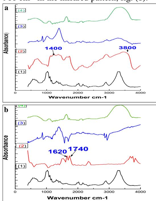
Figure (8) Shows FTIR of the experimental sample which cleaning **a.** Arabic gum by nano gel, **1)** samples before applying stains. **2)** surface of the sample after applying wax stain, **3)** sample after cleaning by nano gel 5%, **4)** standard sample of nano gel, **b.** paraloid B72 by nano gel, **1)** samples before applying stains. **2)** surface of the sample after applying paraloid stain, **3)** sample after cleaning by nano gel 5%, **4)** standard sample of nano gel.
